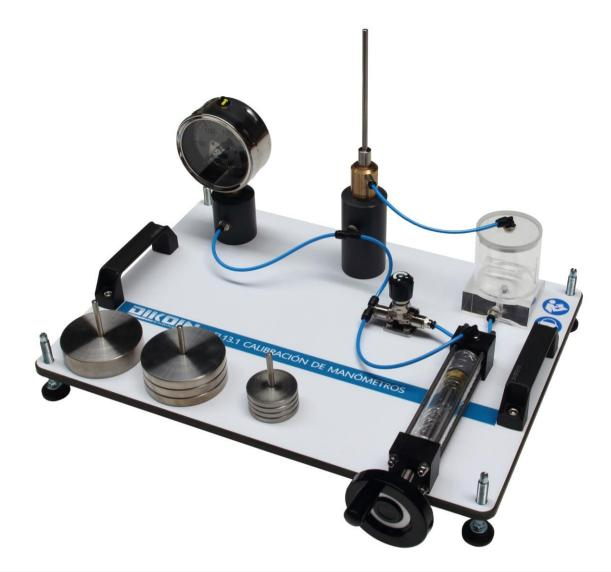
The objective of this equipment is the study and calibration of manometers, as well as the visualization and understanding of its operation.
