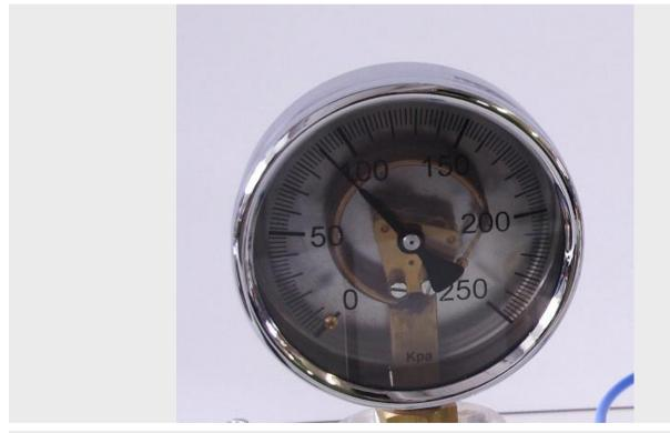
The manometer has the transparent front, in order to show the student the operation of a manometer.
